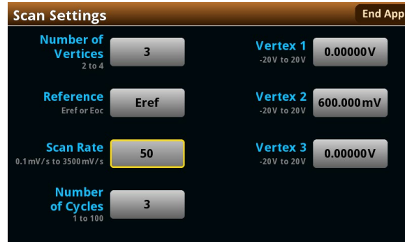
2461-EC Cyclic Voltammetry Test Configuration Screen
