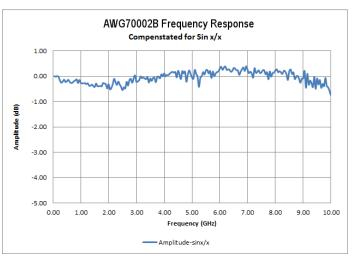
AWG70002B measured frequency response and ideal Sin(x)/x response at 25 GS/s.
