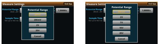
Figure 133: Selecting the Voltage Range
