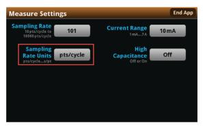
Figure 24: Measure Settings menu, selecting Sampling Rate Units
