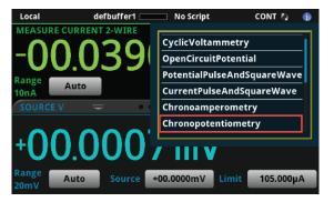
4. Select Chronopotentiometry. The test application begins to run immediately and the following screen is displayed.
