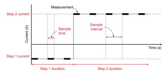
Figure 124: Possible double-step Chronopotentiometry (DSCP) plot
