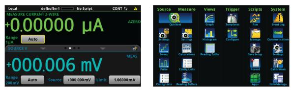
When you run an electrochemistry test application, the default Home and Menu screens are replaced by application-specific Home and Menu screens. These screens vary, depending on the potentiostat or galvanostat test application. You can access these screens with the **HOME** and **MENU** keys. You will see examples of these screens later in this manual.
