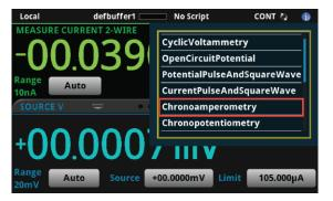
4. Select Chronoamperometry. The test application begins to run immediately and the following screen is displayed.
