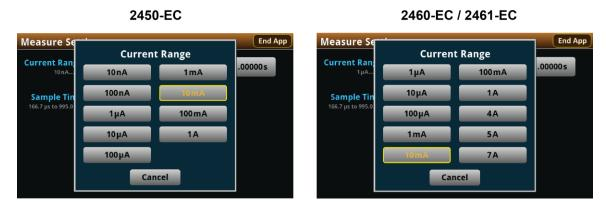
Your instrument will integrate and average the current over the sample time duration. Longer sample times will reduce the effect of noise on the measurement.
