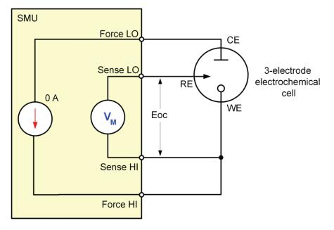
You can use this potential measurement as the zero measurement when defining the voltage vertices. When you do this, the Eoc measurement gets added to the voltage.
