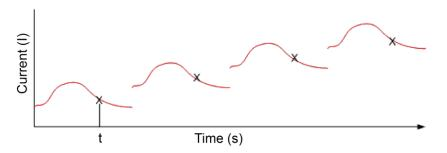
Conversely, the 2450-EC, 2460-EC, and 2461-EC use an internal analog integrator to integrate current over most of the voltage step and report the average current over the aperture time (dt) of the voltage step. See the following figure. This average current is used in the generation of the voltammogram.
