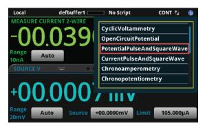
4. Select PotentialPulseAndSquareWave. The test application begins to run immediately and the Potential Pulse and Square Wave home screen is displayed.
