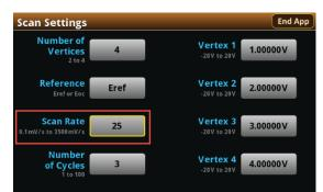
Figure 21: Scan Settings menu, selecting Scan Rate
